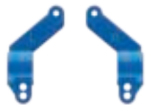
Aluminum axle carriers installed as labeled: 4° toe-in
