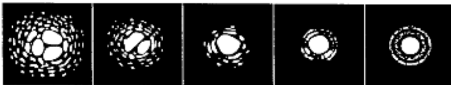
Figure 5-3 Seeing conditions directly affect image quality. These drawings represent a point source (i.e., star) under bad seeing conditions (left) to excellent conditions (right). Most often, seeing conditions produce images that lie somewhere between these two extremes.
