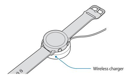
3 After fully charging, disconnect the Galaxy Watch Active from the wireless charger. First, disconnect the wireless charger from the charger and then unplug the charger from the electric socket.
