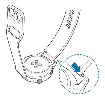
4 Slide the spring bar inwards and connect the new band.
