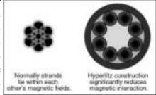
tor. In most cables, the magnetic field of any given strand encounters a complex and changing series of interactions as it travels through a constantly changing magnetic environment. As the magnetic field is modulated, the audio signal becomes confused and distorted.
