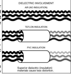
profound effect on an audio or video signal. Dielectric constant, the most often quoted specification for insulating material, is actually not very helpful in understanding the audible attributes of different materials. The coefficient of absorption value is more relevant, and the dissipation factor and the velocity of propagation are even more useful.
