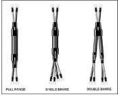
Biwiring within a single cable is a compromise, though often a very practical and cost-effective compromise. Much of the advantage of biwiring is due to magnetically isolating the high and low frequency conductors, and they cannot be isolated quite as well within a single cable.
