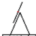
Figure 1 — Combination ladder in standing ladder position with extending ladder at the top
