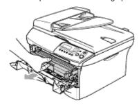
Hold your Brother machine with one hand and hold the drum unit with the other hand. Then, pull the drum unit toward you and lift it up.
