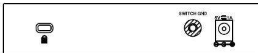
Figure 2– DGS-1100-05 Rear Panel
