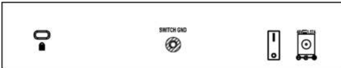
Figure 6 – DGS-1100-08P Rear Panel
