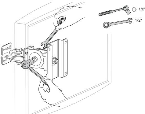
Side-to-Side Motion Move monitor side-to-side through entire range of motion. If it does not stay in place at any point it will need adjustment - see below. Adjust so side-to-side moving forces are equal.
