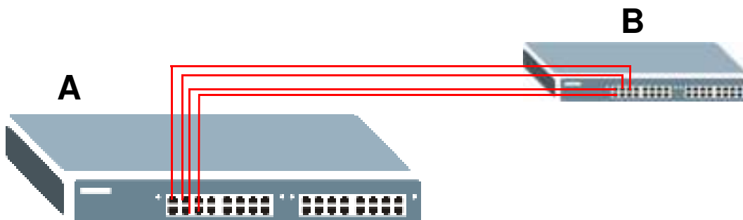
Figure 122 Trunking Example - Physical Connections
