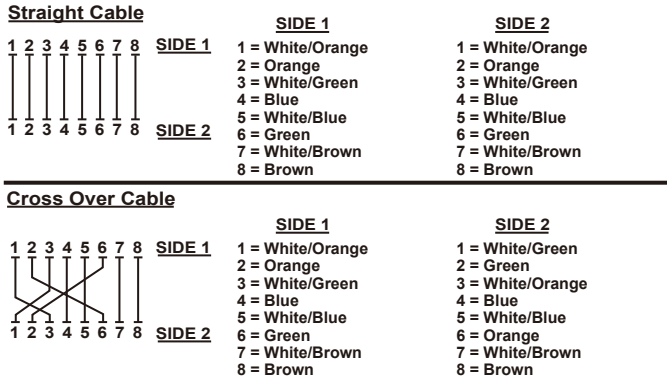
Figure A-1: Straight-Through and Crossover Cable
