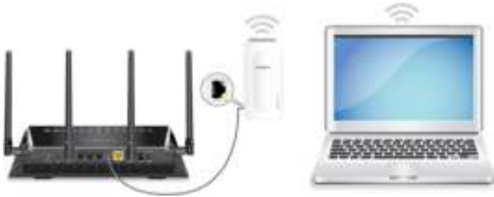
Figure 4. Extender in access point mode
