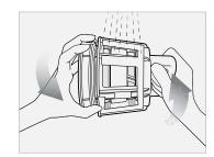
Thoroughly rinse the inside and outside of the strainer under running water.
