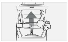
Remove the juicing screw, strainer and rotation wiper unit from the juicing bowl. Clean with provided brush.
