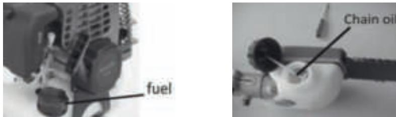
1. Feed fuel into the fuel tank and tighten cap securely. For pole chain saw, feed chain oil into oil tank.
