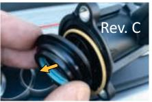
Pull on the diaphragm shroud (revision G), or the plastic "basket" (revision D), and the whole assembly will pop off leaving the bare solenoid coil. For revision C, first pull the piston from the body and remove the spring. Then remove the piston shroud - this can usually be pulled out by hand, but if it's too tight, it can be carefully levered out with a flat screwdriver. The thin plastic may be damaged, however it is not reused in the VTA installation.
