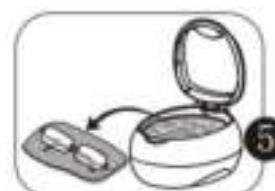
The unit will stop automatically after 3 minutes. If another cleaning is needed, press the ON button again.
