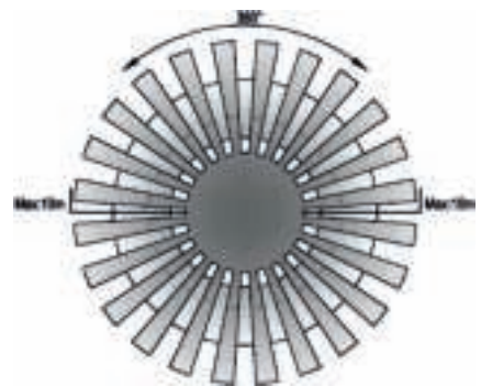
6. Detection distance: max. 20 meters.
