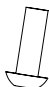
15 M4*10 Hexagon flat round head screw x2 内六角平圆头螺丝M4*10
