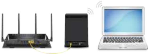
Figure 5. Extender in access point mode
