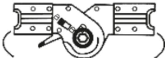
The hinges click into place automatically when unfolded.
