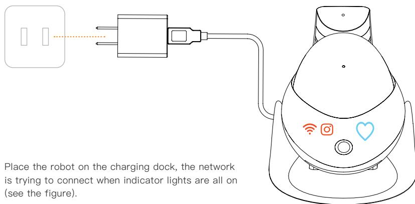
Place the robot on the charging dock, the network is trying to connect when indicator lights are all on (see the figure).
