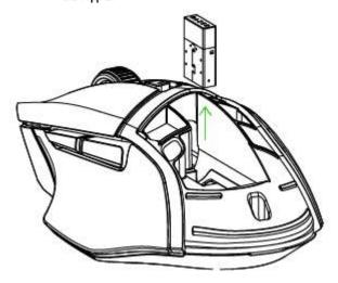
5. Close the top cover and connect the wireless USB dongle to the USB port of your computer.
