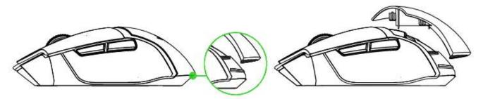
Insert the included AA battery into the Razer Basilisk X HyperSpeed following the directions indicated on the battery compartment.
