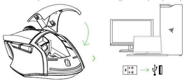
6. Switch the slider to 2.4 GHz mode. The status indicator will start blinking rapidly.
