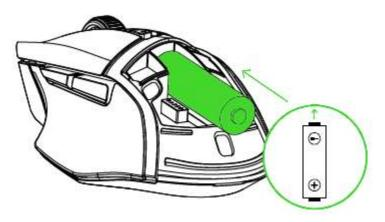
Caution: The included AA battery is non-rechargeable. Dispose of this battery in accordance with your local environmental laws. For your safety, only use an alkaline battery.
