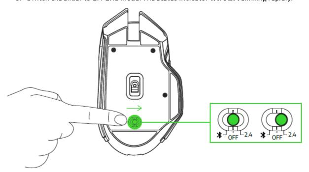
7. Wait until the mouse automatically pairs with the wireless USB dongle. When paired, the status indicator will change to static blue for 5 seconds before turning off.
