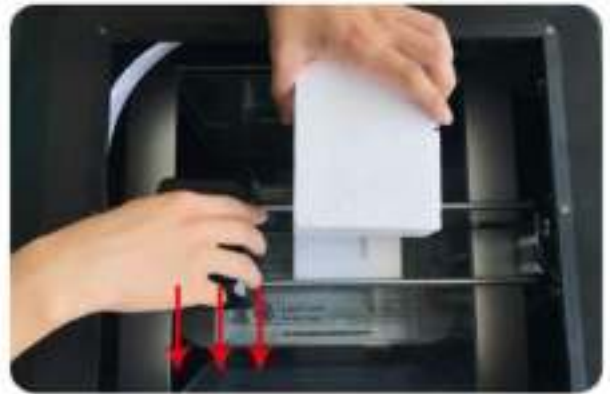
10. Move extruder to the front side and take out the foam.
