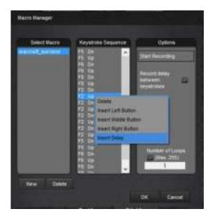
Up to 12 macros can be stored within the Macro Manager. The maximum number of keystrokes is 62, plus mouse commands and delays. Please note, pressing and releasing a key represents two commands. Assign each macro to a mouse button through the "Button Assignment" menu (see 9.11 Button Assignment).
