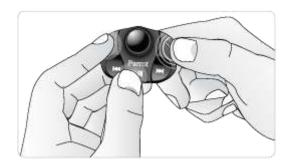
After verifying the CR2032 battery is properly inserted in the remote unit, press and hold the the and buttons then press the button several times. This has to be done during a 30 seconds period once the ignition is turned on.
