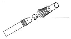
• Loosen the knobs at the search coil's end, then adjust the search coil to the desired angle. (The search coil should be parallel with the ground.) Tighten the knobs just enough to keep the search coil from rotating or wobbling.
