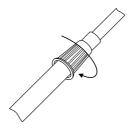
• Then turn the stem's lock nut counter clockwise to lock it in place.
