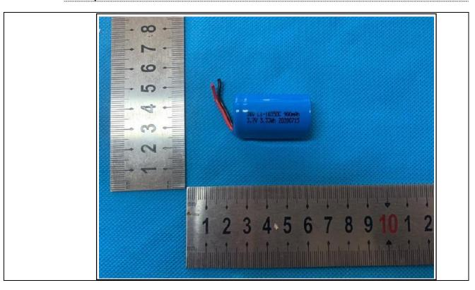
Battery ICR 14500 600mAh 3.7V Details of:
