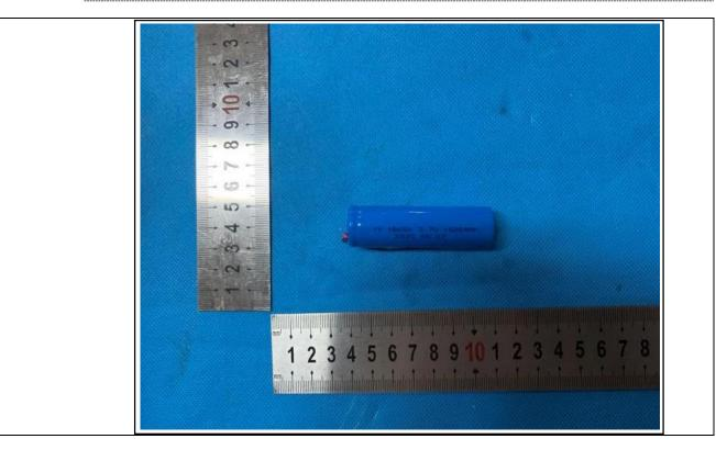
Details of: ICR 18650 2600mAh 3.7V
