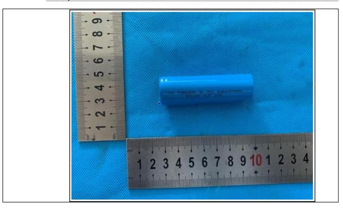
Details of: Battery ICR 18650 2500mAh 3.7V
