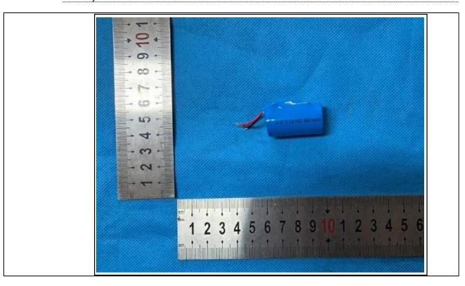
Battery CKH 18350 900mAh 3.7V Details of:
