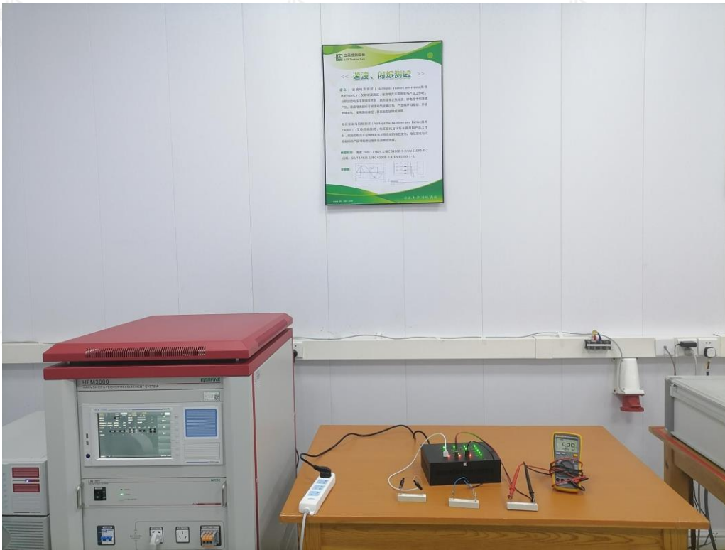
Test Setup Photo of Harmonic & Flicker Measurement
