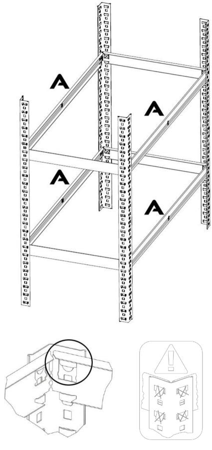
**Step 3**. Connect the middle beams: C
