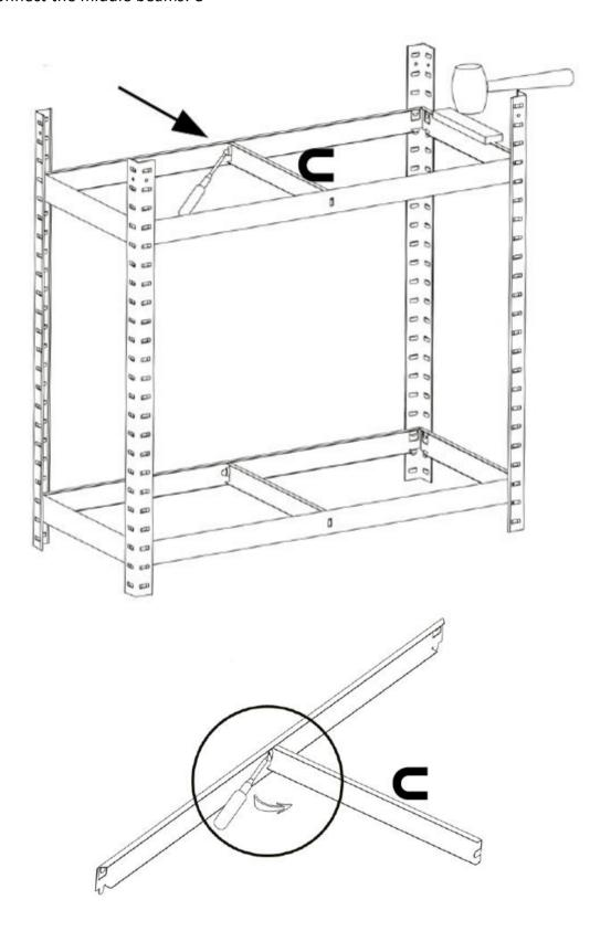
**Step 4**. After finish bottom part, add connector: E Then add: F,B,A,C
