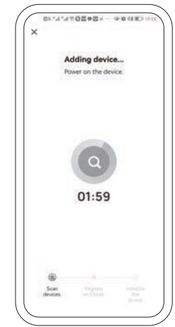
B4.7. After clicking "EZ mode", the application will search for smart devices in the same WiFi environment by itself. Meanwhile pay attention to the tips.
