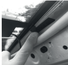
Stick the transparent part of the antenna on the windshield and put the black part on the metal frame.
