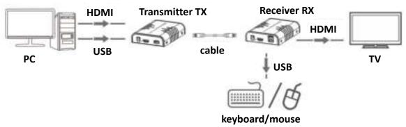
NOTE: Point to multi-point connection via switch is supported too, but under point to multi-point configuration, it is strongly recommended to operate KVM function on one receiver only at the same time.
