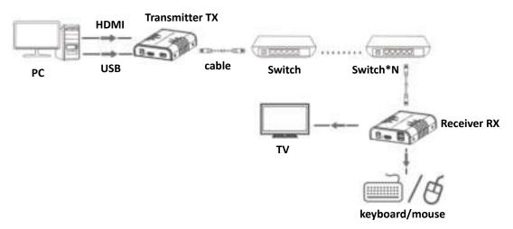
**NOTE:** Transmission distance depends on type of network cable, CAT5: 80m, CAT5E: 100m, CAT6: 120m.
