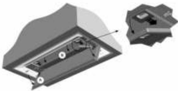
Take hold of the right and left side of the plate (a) and pull down simultaneously.
