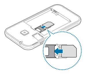
▶ **Dual SIM models**: Insert the SIM or USIM card with the gold-coloured contacts facing downwards.
