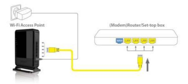
Connect the supplied power-adapter to the power inlet port and connect it to a wall outlet. Switch the access point on by flipping the switch on the back of the device. The access point automatically enters the self-test phase. During self-test phase, the Power LED will be lit continuously to indicate that this product is in normal operation.
