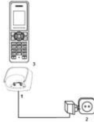
Figure 6: Setting up the charger station
