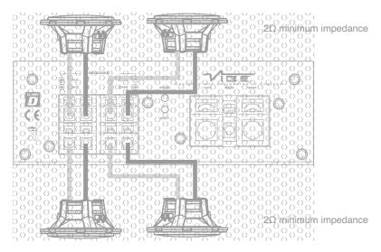
Bridged Wiring Configuration
