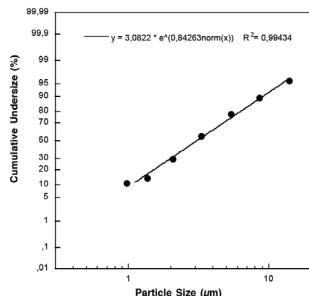
Measurements were performed using a sodium fluoride solution with a "Next Generation Impactor" (NGI). The diagram may therefore not be applicable to suspensions or highly viscous medications. You can obtain more detailed information from the manufacturer of your medication.
