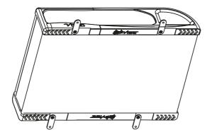
Step 2: Secure the enclosure with four screws.
