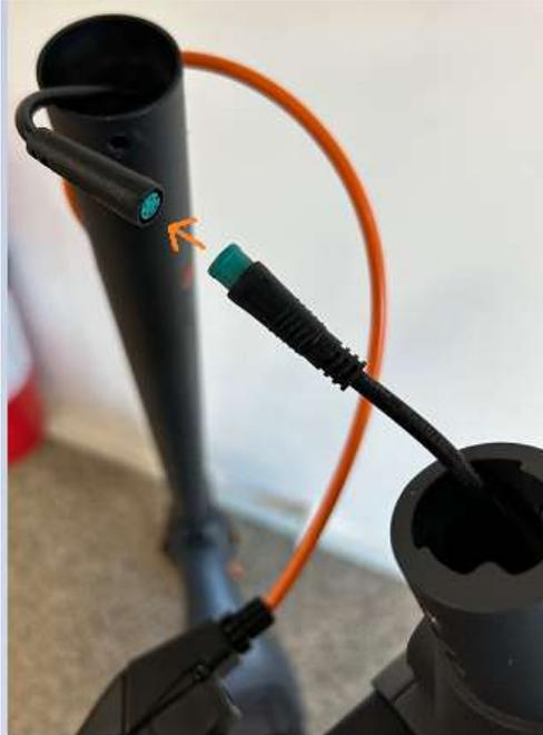
2. Lower the cable inside the tube and carefully lower the steet without getting the cable stuck.
