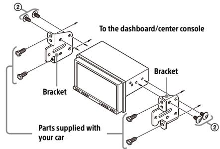
When mounting this unit to the preinstalled brackets of your car, use the mounting screws ② in the appropriate screw holes based on your car: T for TOYOTA and N for NISSAN.
