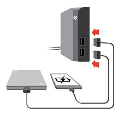
Backup Plus Hub's additional USB ports allow you to connect more devices to your computer. Simply connect compatible USB devices to the two USB Type A ports on the Backup Plus Hub. When Backup Plus Hub is connected to your computer, the devices are also available to the computer.
