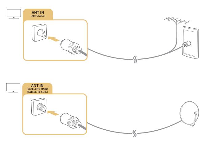
It is best to connect the both connectors using a Multi-Switch or DiSEqC. Switch, etc and to set **Aerial Connection Type** to **Dual Oscillator**.
