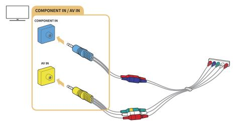
To use component equipment, connect both a component cable(blue) and an AV cable (yellow).
