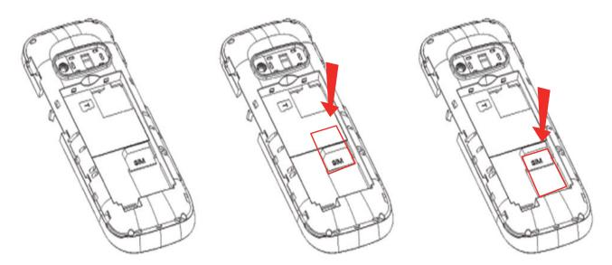
Above the SIM card slot on the right side, there is the slot for a microSD memory card. Slide the pin right and then lift it upwards. Insert the microSD card making sure that the microSD card contacts are connected with the phone's terminals, close the pin and slide it left.
