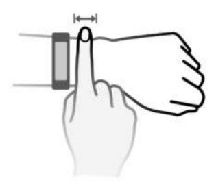
The watch strap adopts a U-shaped buckle design so it won't fall out easily. To wear the watch, insert one end of the strap through the U-shaped buckle and then fasten it. The end of the strap is intentionally bent so as to enhance wearability.
