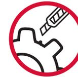
EN Burrs on the jumper should be gently grinded with the emery paper or carefully cut with the stationary knife.
