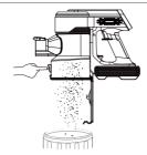
• Press vertically the dust cup release button of the main body, grasp the bottom of the dust cup, and take out the dust cup.
