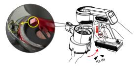
**Note**: The function of the air filter element is to allow the device to dissipate heat and dredge the air more effectively during operation, without frequent cleaning. If necessary, press the air filter release button to remove the air filter.
