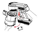
• Pull out the HEPA filter. Then open the bottom cover of the dust cup, rotate the stainless steel filter and take it out.
