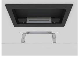
Then, by continuously sliding the two handles outwards, move the cover over the burner and cover the opening from which the flame is coming. This should be done evenly and simultaneously for the entire width.
