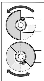
Place the protective guard (7) on the spindle collar. Adjust the position of the protective guard (7) to meet the requirements of the operation. Lock the protective guard (7) by tightening the locking screw (6) using the hex key (3).
