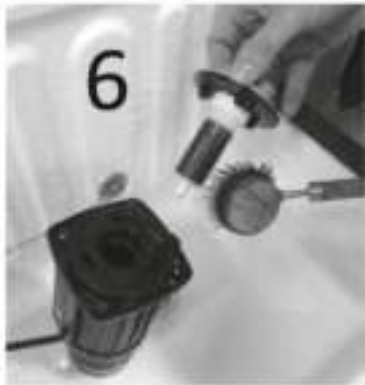
Clean rotor with water and brush
