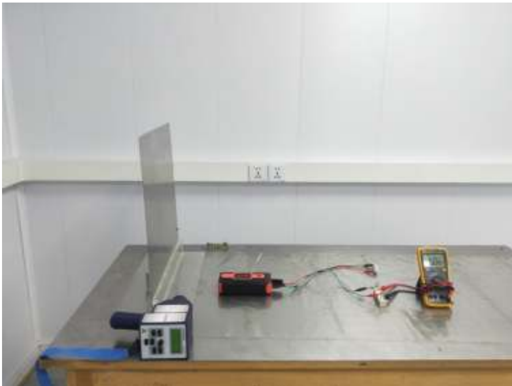
Test Setup Photo of Electrostatic Discharge Test
